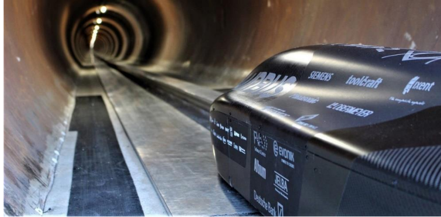
Figure 1.3 Contest pod travelling through the test tube [22]
