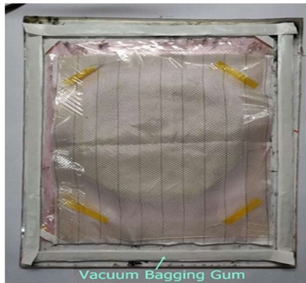
Figure : Vacuum Sealing the specimen using Gum
