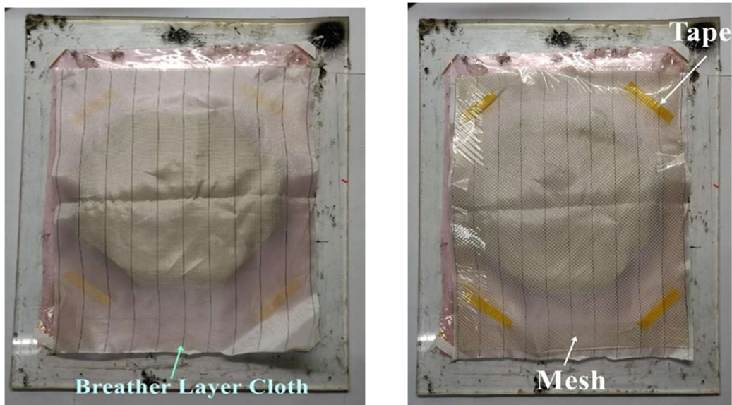
Figure : Attaching the Breather Layer Cloth and the Mesh
