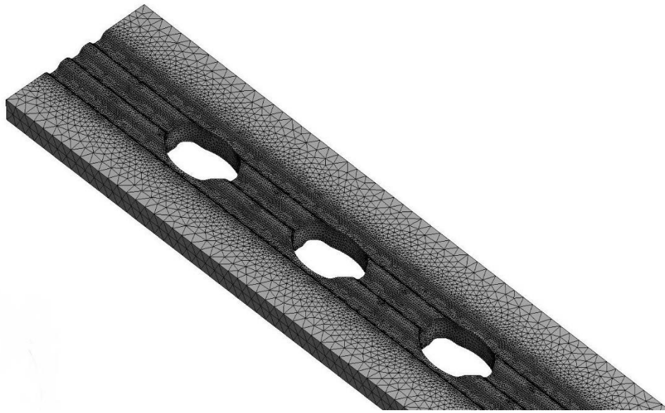
a) Isometric view of mesh generation in three corrugated fin
