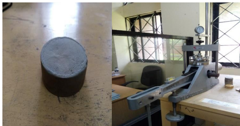
Figure 3.11. Oedometer test with sample
