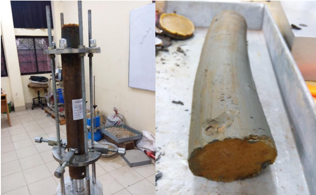
Figure 3.3. Sample extraction from Shelby tube
