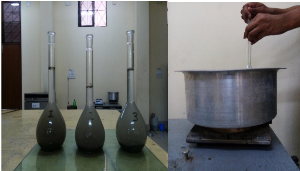
Figure 3.5. Laboratory test of determination of Specific gravity of soil.
