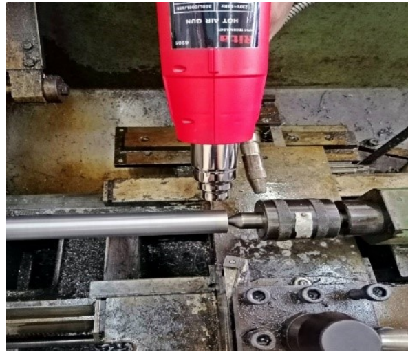
Figure 12: Heating Work piece with a Hot Air Gun
