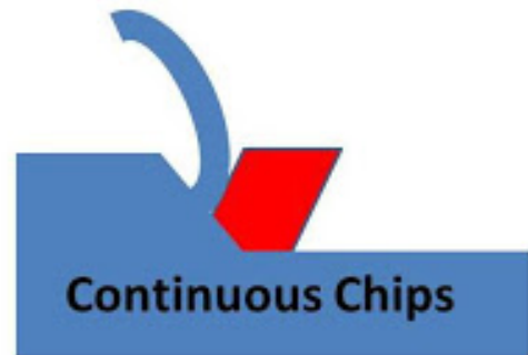
Figure 16: Schematic Diagram of Continuous Chips [9]
