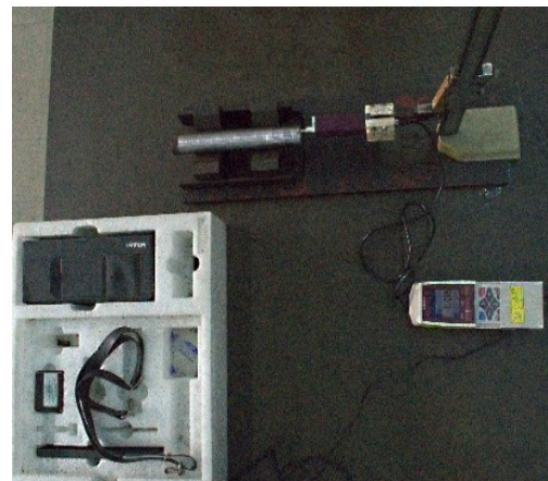
Figure 7: Profilometer setup for measuring surface roughness (Mitutoyo SurfTest SJ-210-Portable Surface Roughness Tester)
