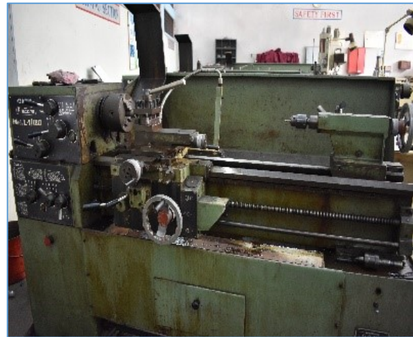
Figure 3: Horizontal Central Lathe (Gate Pinacho Mod. L-1/180)
