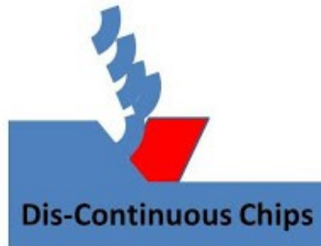
Figure 17: Schematic Diagram of Discontinuous Chips [9]
