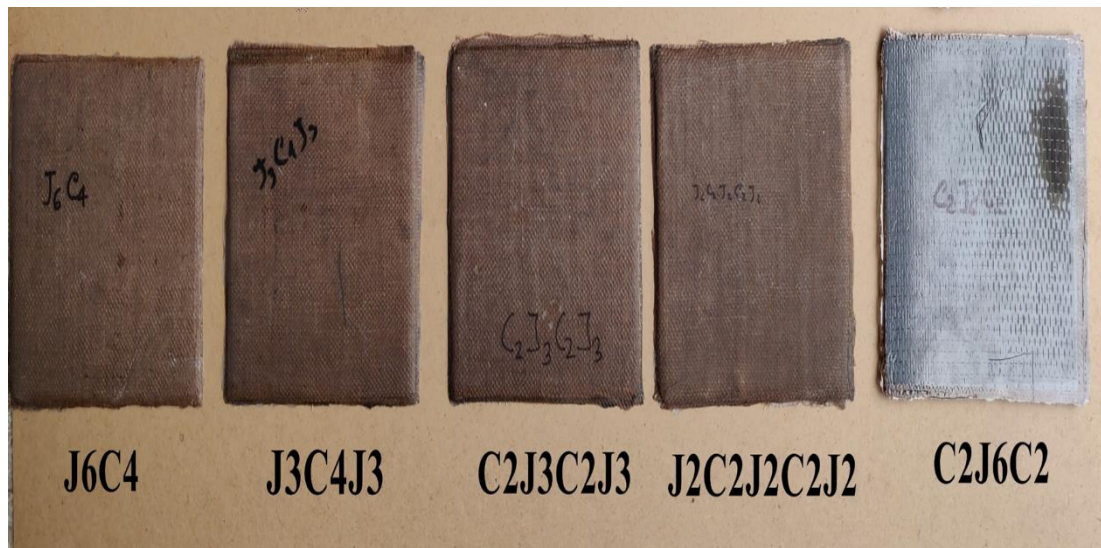
Figure 9: Infused Hybrid Composites with Five Different Stacking Sequence
