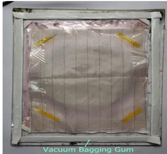
Figure 7: Vacuum Sealing the specimen using Gum
