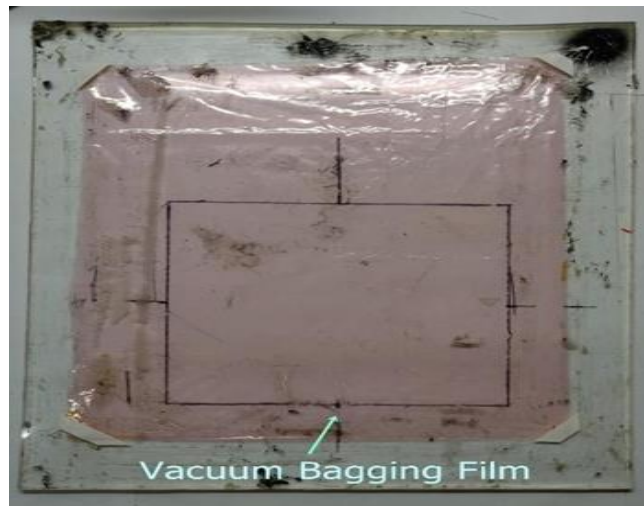
Figure 3: Acrylic Glass as Mould
