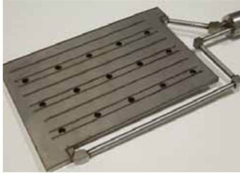
Figure 3.18: Stainless steel collector after laser welding[37]
