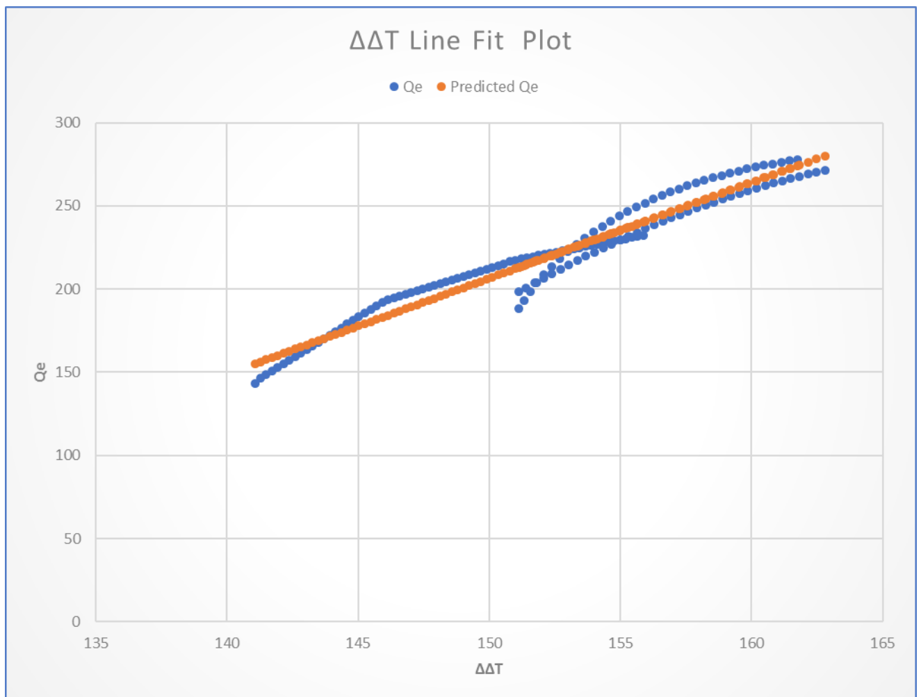
Figure 6.7: Line Fit plot showing the predicted cooling capacity versus the actual cooling capacity against the arbitrary temperature difference function
