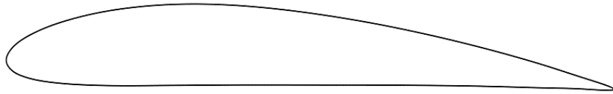
FIGURE 33: NACA 4412 AIRFOIL PROFILE
