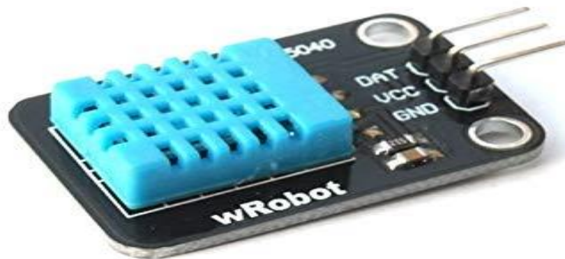
Figure 3.6 DHT11 (Temperature and Humidity) sensor
