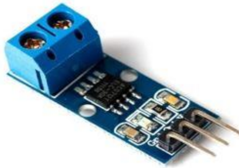
Figure 3.4. ACS712 Current Sensor
