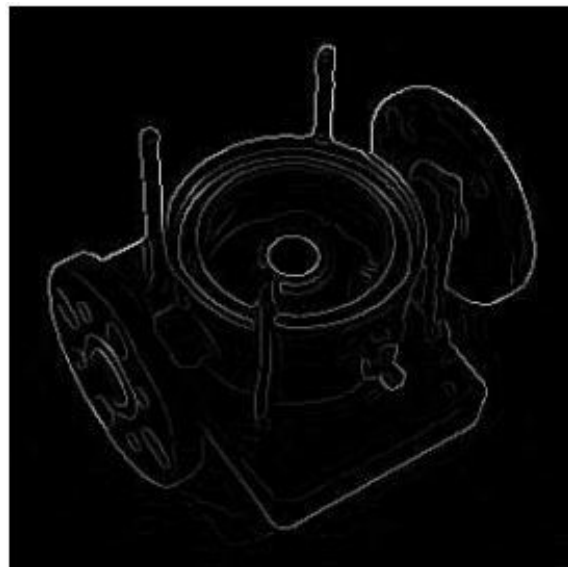
Fig. 3.9 Non-Maximum Suppression with Interpolation[36]
