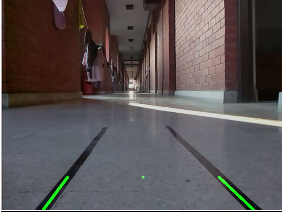
Fig. 5.4 Lane and Current position Detected Frame
