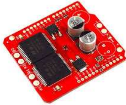
Fig. 4.4 VNH2SP30 full-bridge motor driver
