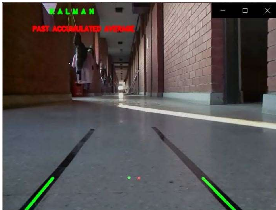
Fig. 5.5 Past Accumulated Average method Vs Kalman Filter Algorithm
