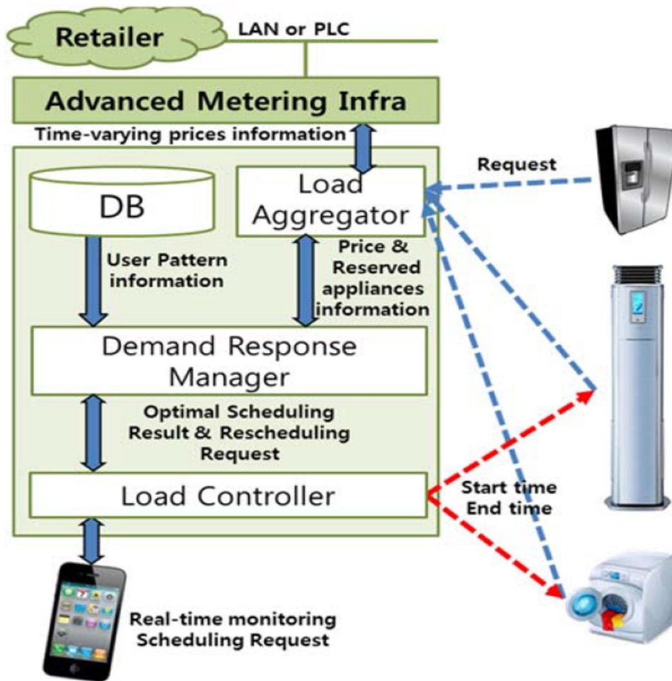
Figure 2.4: Use of AMI & PLC in DSM for real-time monitoring scheduling
