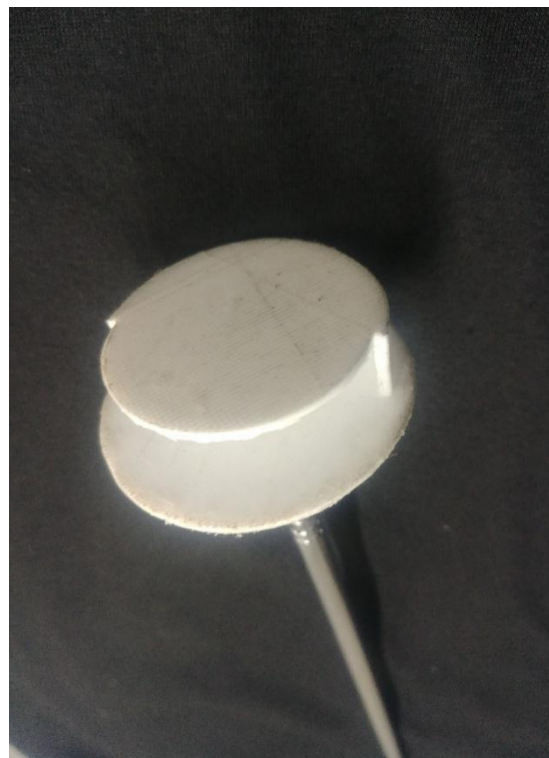
Figure 17: 3D Printed Magnet Casing
