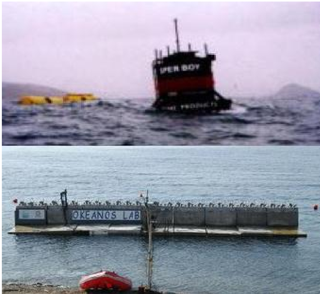
Figure 7: Different concepts of oscillating water columns - Sperboy (above) and REWEC-3 (below) [21]
