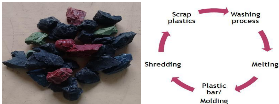
Figure 3.4 Plastic aggregate (Polypropylene) and its preparation process
