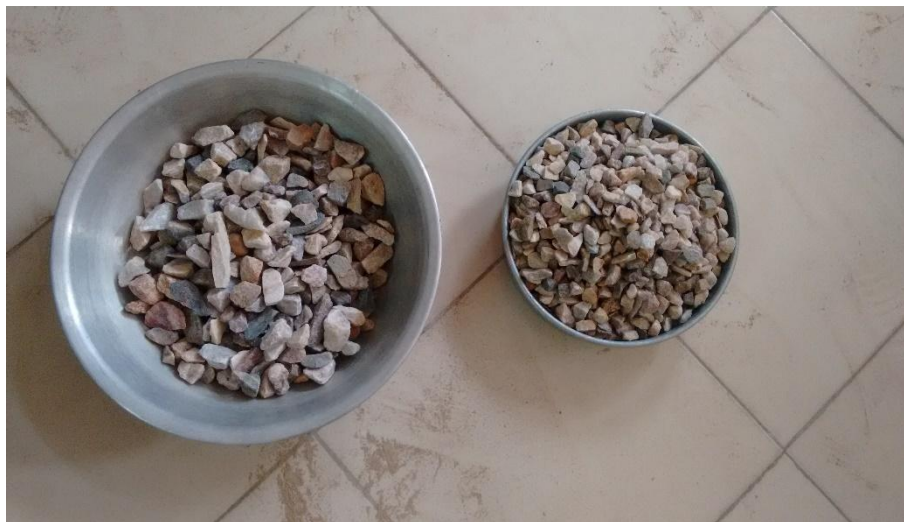
Figure 3.2 Stone chips (crushed)
