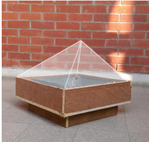
Figure 3.3: Constructed Pyramid Solar Still
