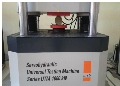
Photo 3.20 Tensile Strength Test
