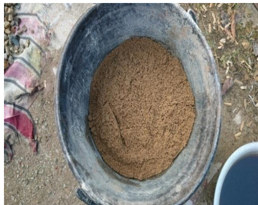
Photo 3.4 Sand After Sieved And In SSD Condition
