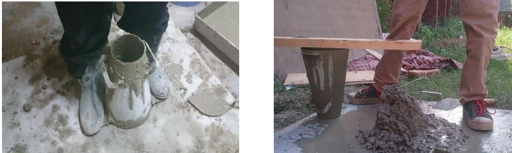
Photo 3.8 Slump Test Procedure at 15 Minute Interval
