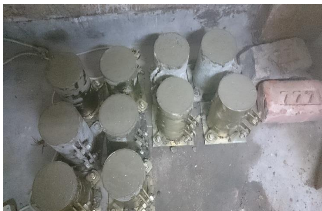
Photo 3.14 Prepared Specimen Casted in Molds
