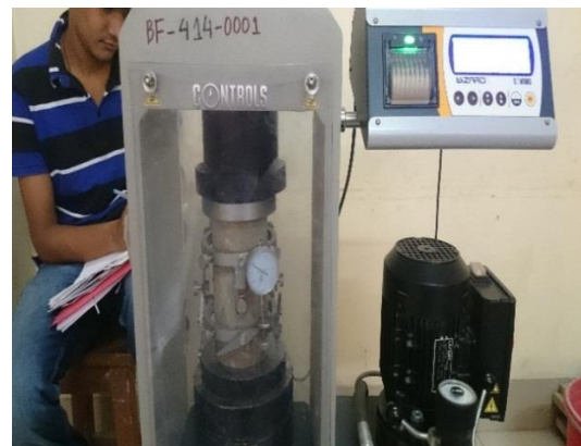
Photo 3.19 Compressive Strength Test
