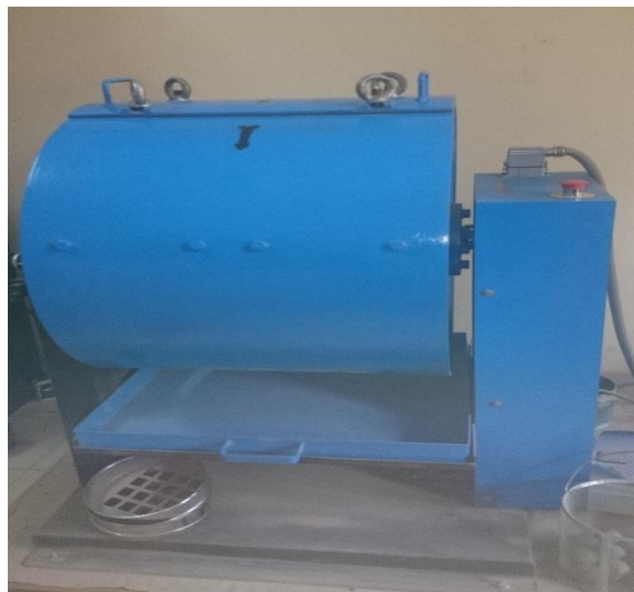
Photo 3.1 Los Angeles Abrasion Test
