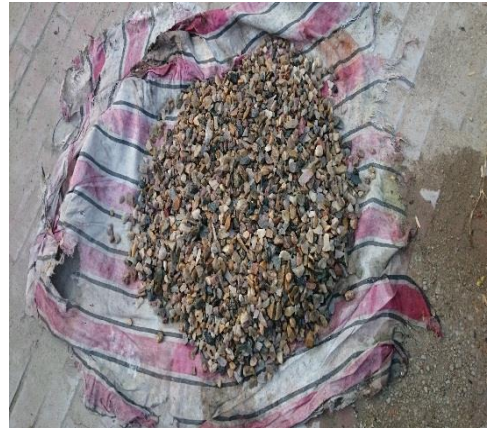
Photo 3.6 Coarse Aggregate SSD Condition
