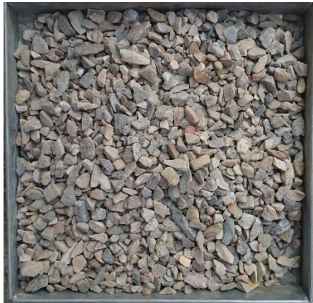
Photo 3.5 Coarse Aggregate Before After SSD Condition
