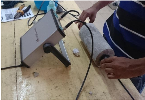
Photo 3.17 Ultrasonic Pulse Velocity Test (UPV)
