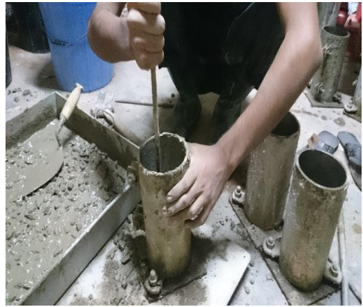
Photo 3.11 Tamping of Concrete
