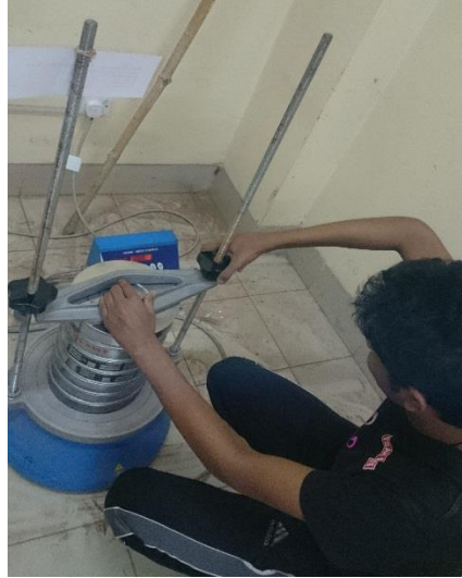
Photo 3.2 Sieve Analysis of Sand for FM Calculation
