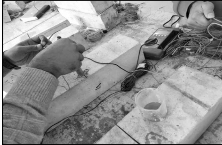
Fig. 3.11. Half-Cell Potential Measurement Using Cu/CuSO 4 Solution
