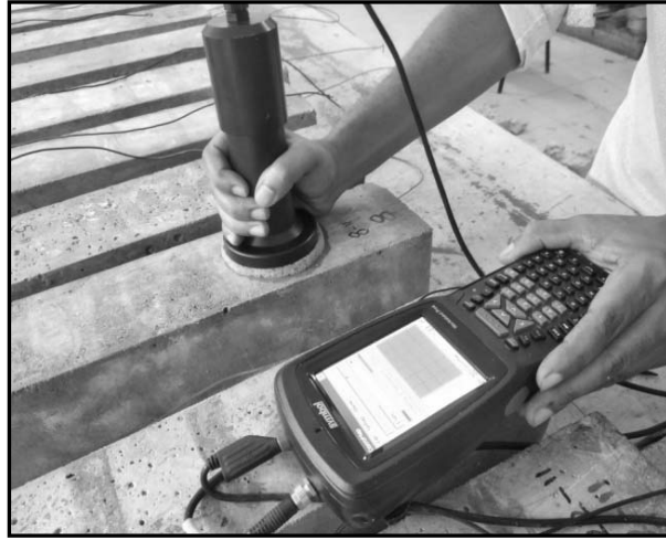
Fig. 3.12. Concrete Resistance Measurement
