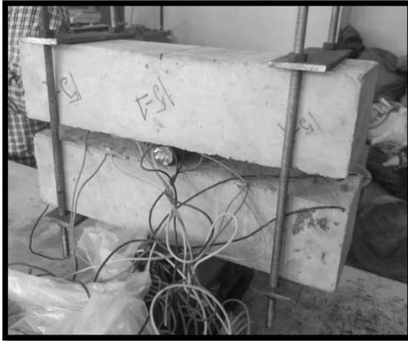
Fig. 3.8. Anchoring of Specimens
