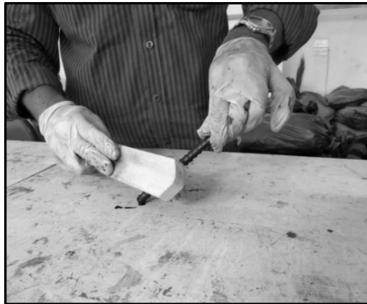
Rubbing Steel Bars with Wire Mesh
