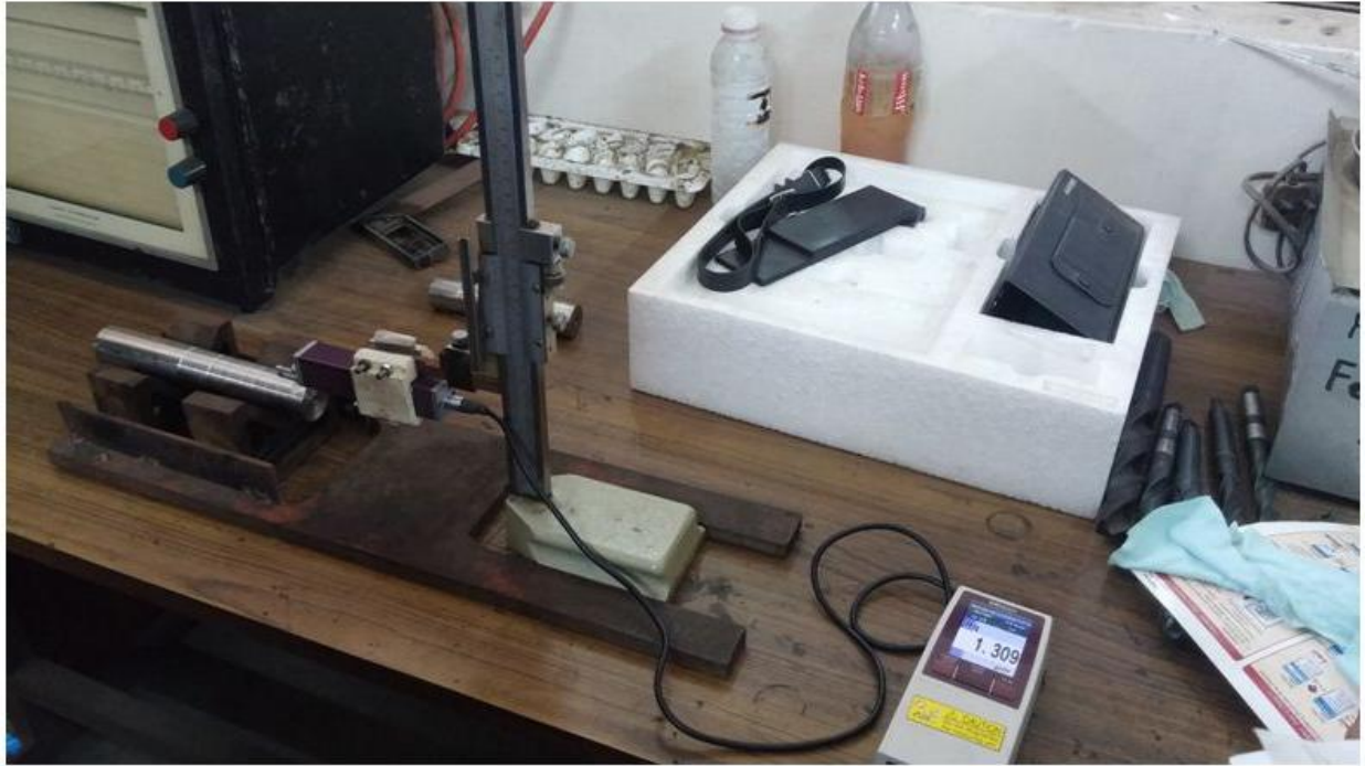
Fig 3.5: Measuring the surface roughness with Mitutoyo surface roughness tester
