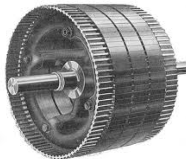
Fig.1.2: Rotor of a squirrel cage Induction Motor [2]
