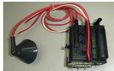
Figure 3.9: A typical TV flyback transformer
