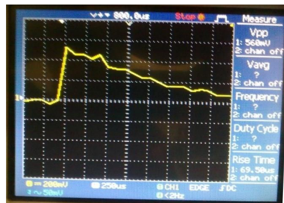
Figure 5.4: Discharge pulse through a 100 \Omega load
