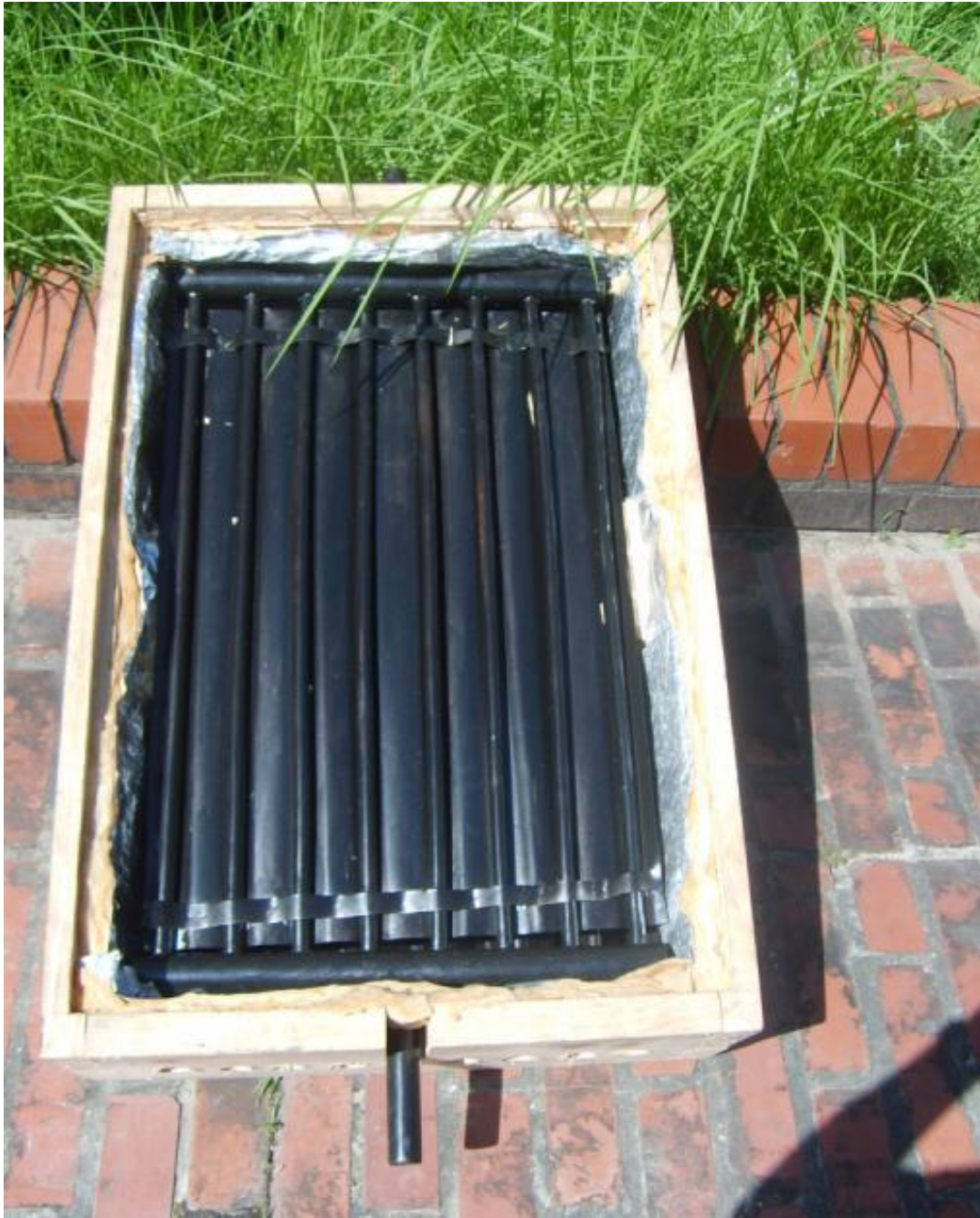
Fig 3.3: Internal constructional view
