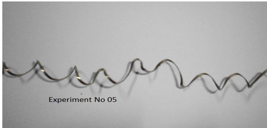
Figure4.14: Chip that we found from the experiment 05
