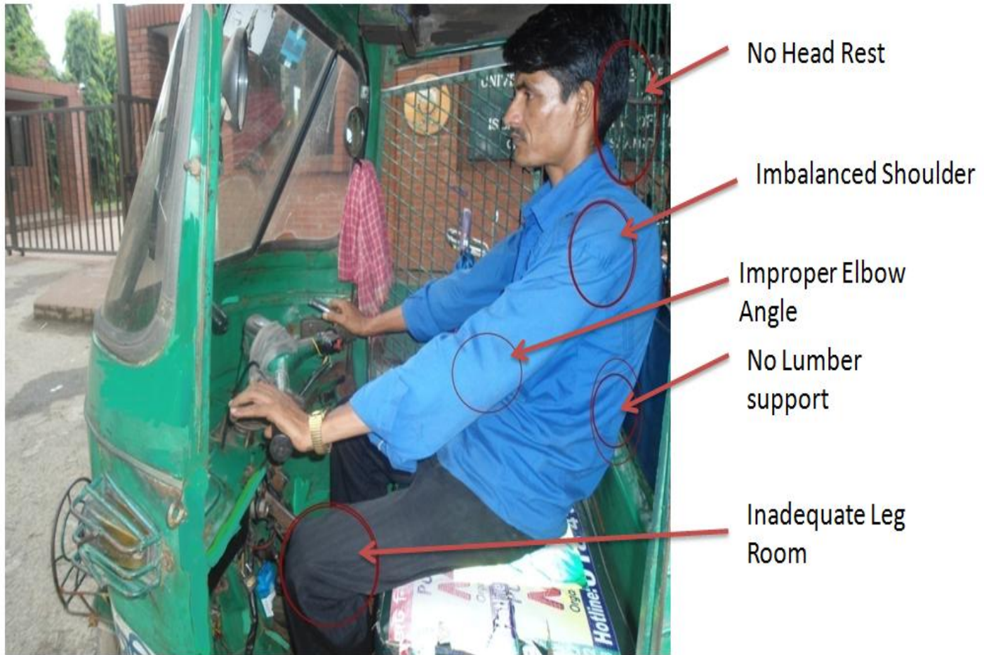
Figure 10: Design Problem in Traditional Vehicle
