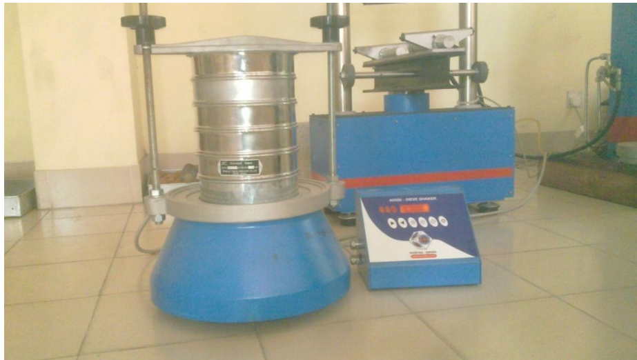
Figure: 2.1 Sieve Shaker Apparatus
