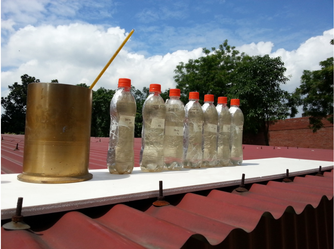
Figure 3.1: Exposing samples into the sun.
