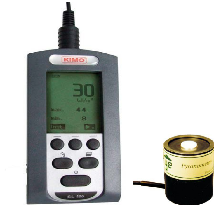
Figure 3.5: Equipment's used in the experiment a Pyranometer.
