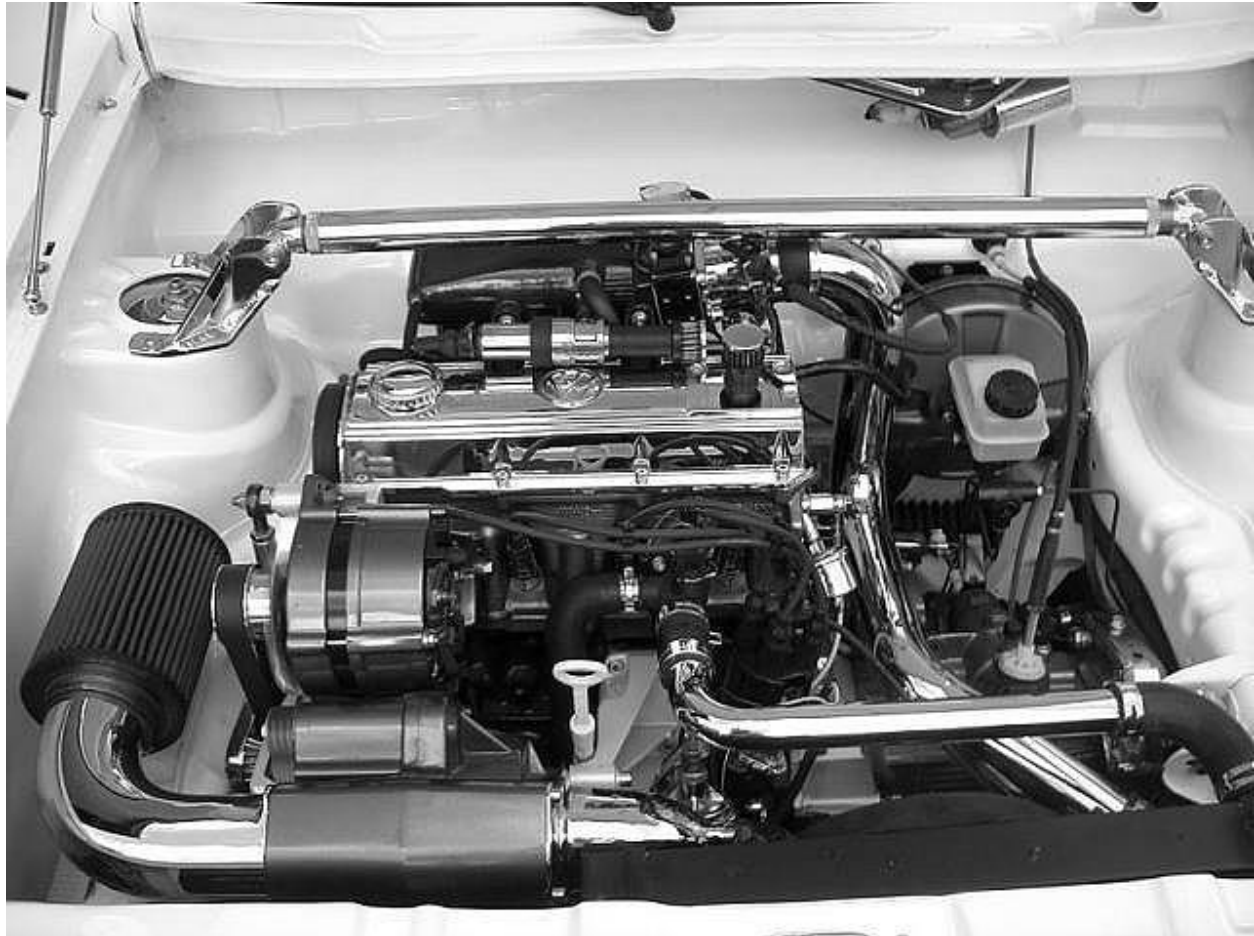
Fig 1.3 : A G-Lader scroll-type supercharger on a Volkswagen Golf Mk1.
