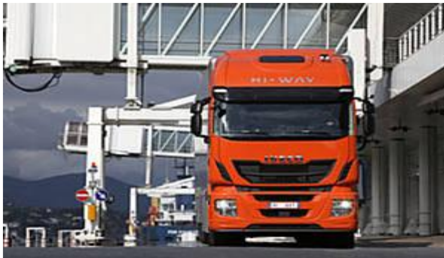
Figure: 1. 13: The truck of the year 2013, Iveco is equipped with anLDWS. In addition, the heavy-duty, long-haul truck implements ACCand ESC functionality as well as an AEBS
