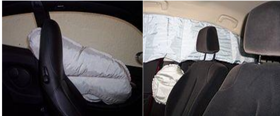
Figure: 2.5a: (left) Side airbag inflated permanently for display purposes, and(right) deployed curtain airbag and side torso airbag in a Citroën C4
