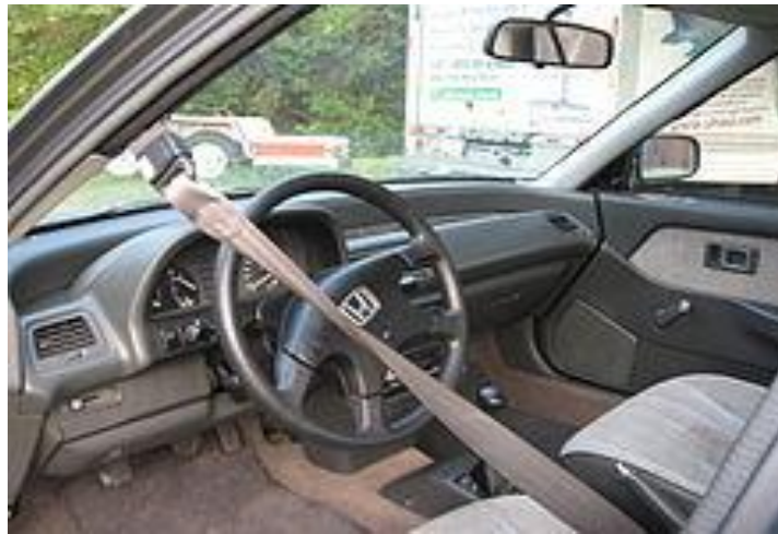
Figure 2.20: Automatic seat belt in a Honda Civic
