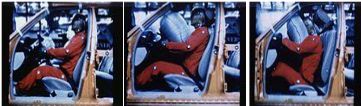
Figure: 2.4.Demonstrating the steps in using airbag
