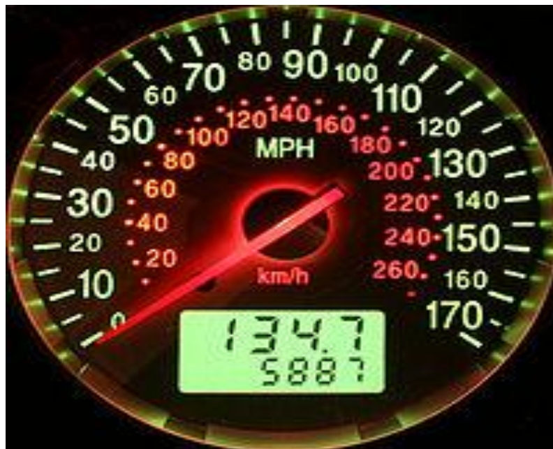
Figure 2.12b: A speedometer showing mph and km/h along with an odometer and a separate "trip" odometer (both showing distance traveled in miles)
