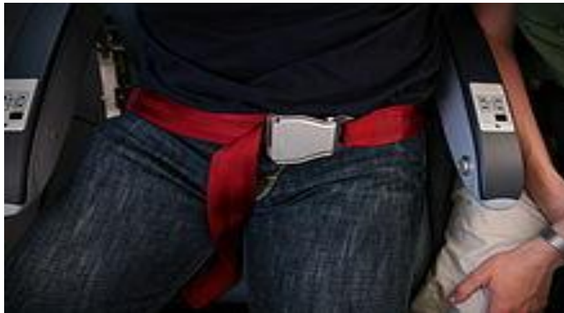
Figure: 1.17: A lap ("2-point") belt in use
