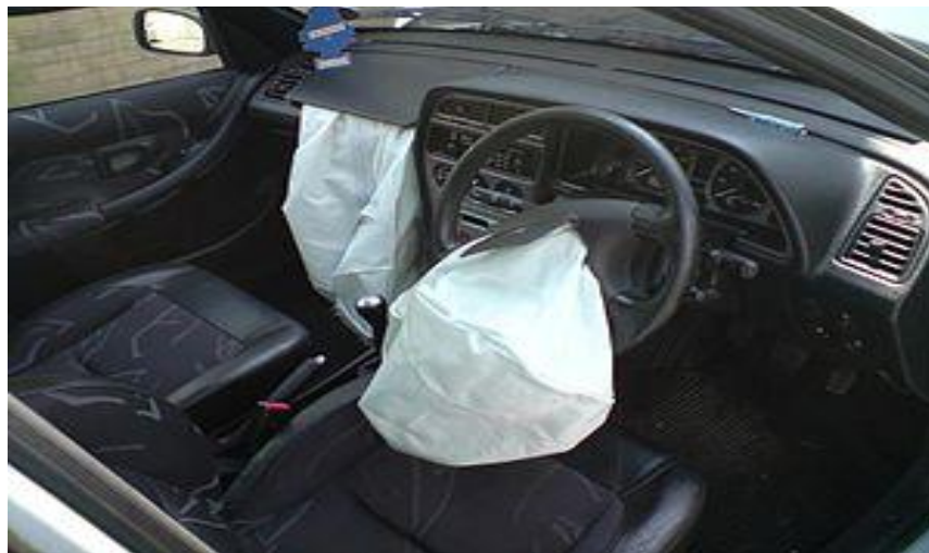
Figure: 2.2: The driver and passenger front airbags, after having been deployed, in a British Peugeot 306 car.
