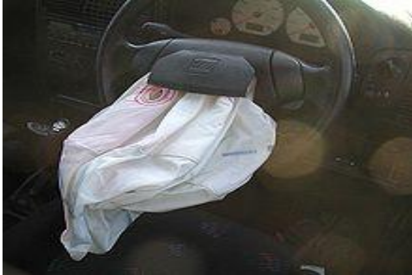
Figure: 1.10: Post-deployment view of a SEAT Ibiza airbag
