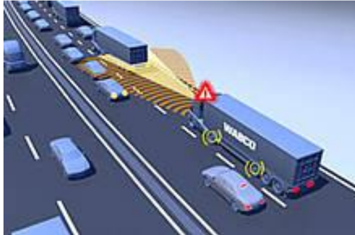
Figure: 2.15: The On Guard Max system by Wabco reacts to moving and stopped vehicles
