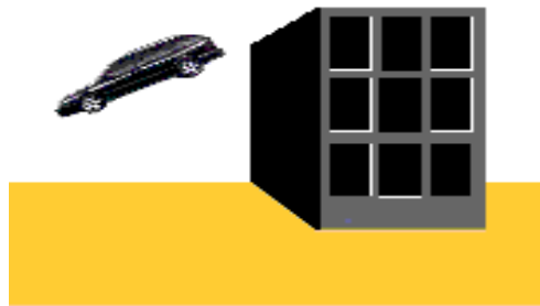
Figure: 31. (a) Dropping off 3 storey building is equivalent to crashing at 50km/h
