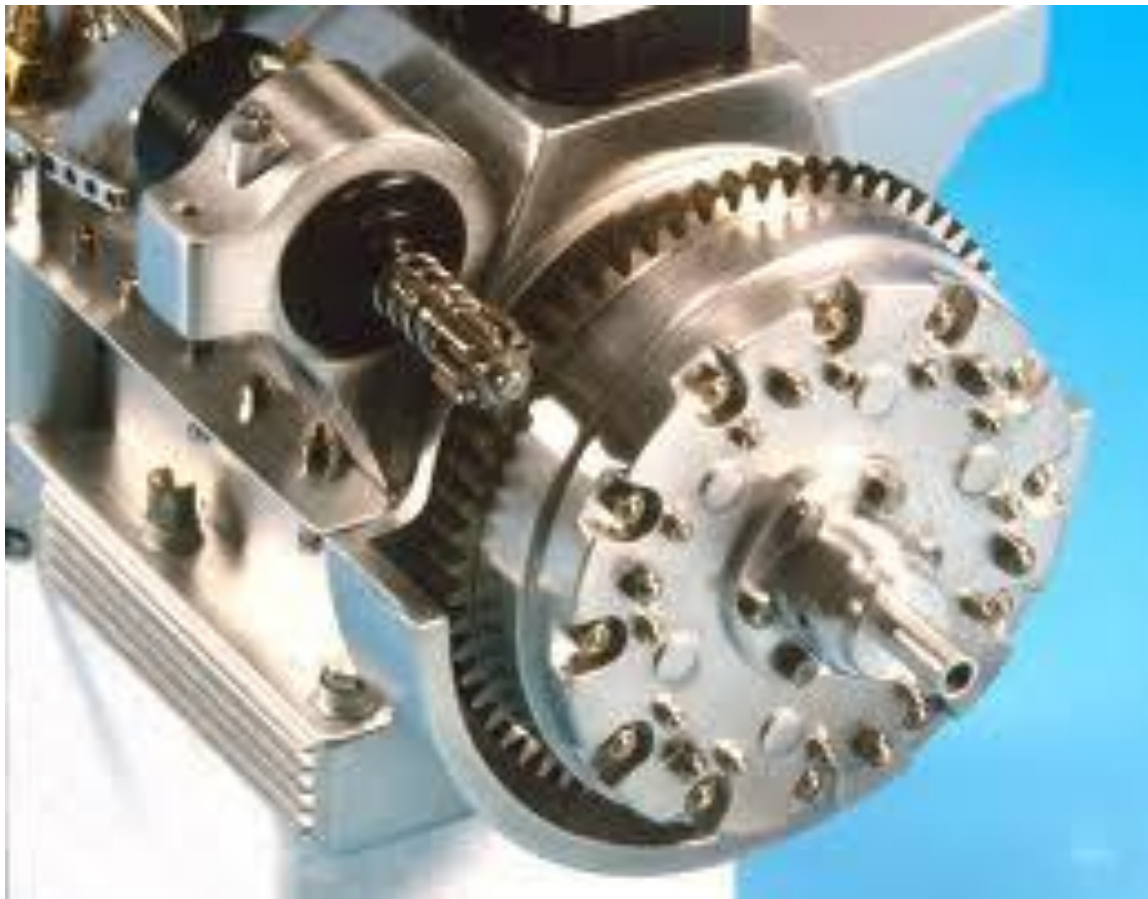
Fig: 3.18 Pinion of Starter Motor with Flywheel [24]
