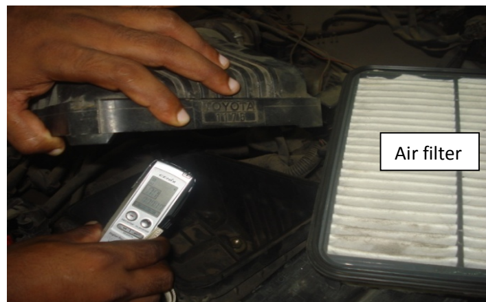
Figure:4.2.c- Sound recorded with air filter and without use air filter.
