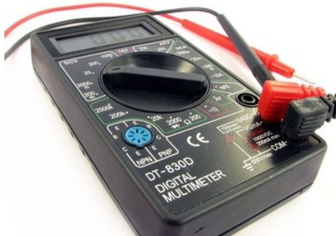
Fig: 2.B -A digital multimeter will help diagnose problems with the fuel injectors in the vehicle.
