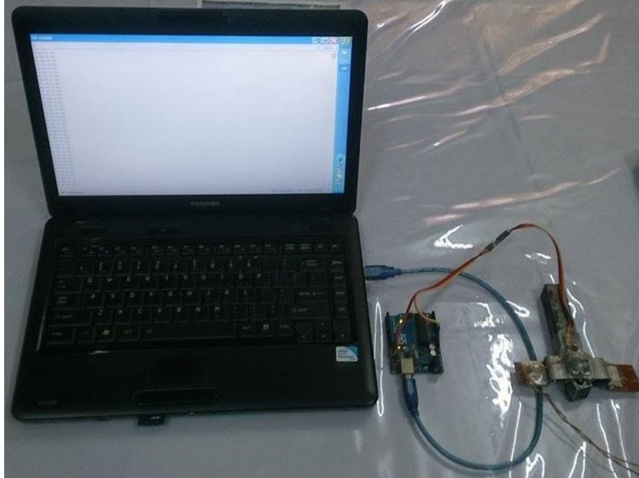
Figure 3.29: Photograph of the setup of the accelerometer for measuring the vibration of the tool holder and the cutting tool
