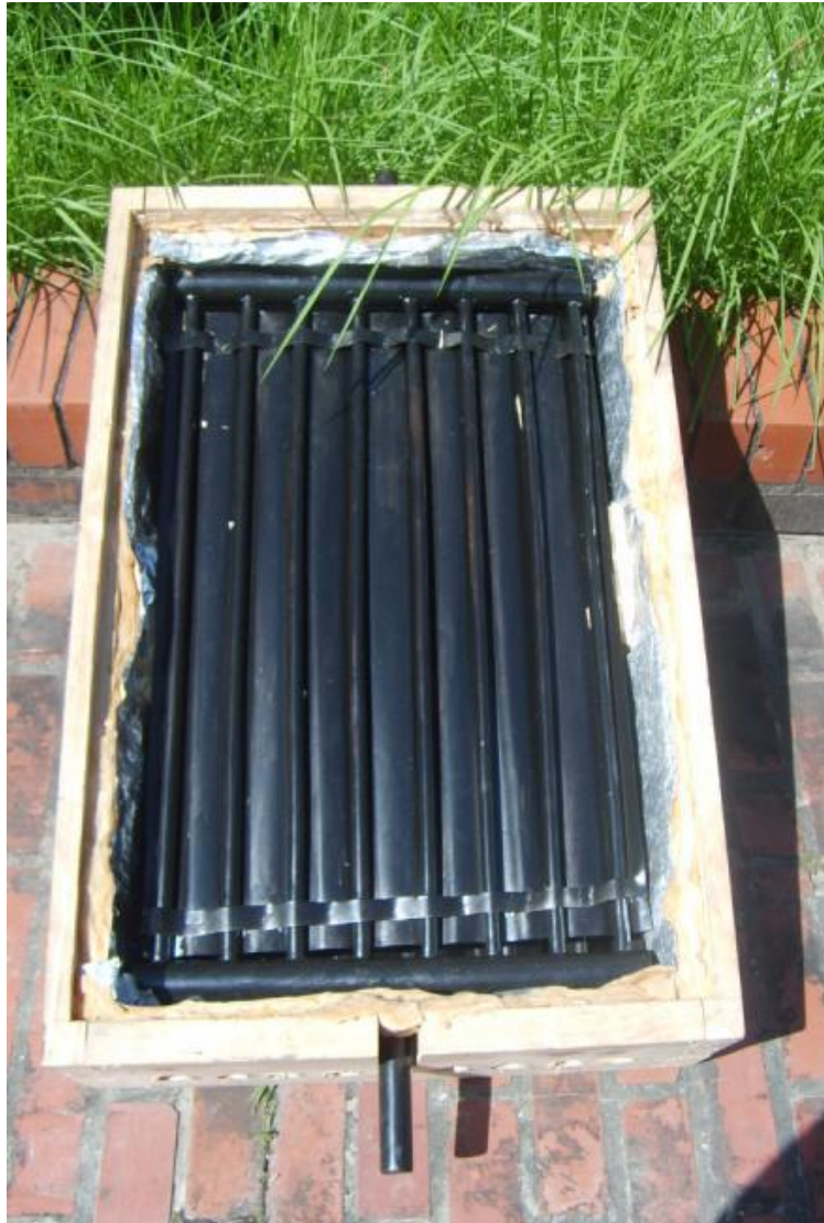
Fig 3.4 Photograph of the Interior view showing the TMS with water heat exchanger.
