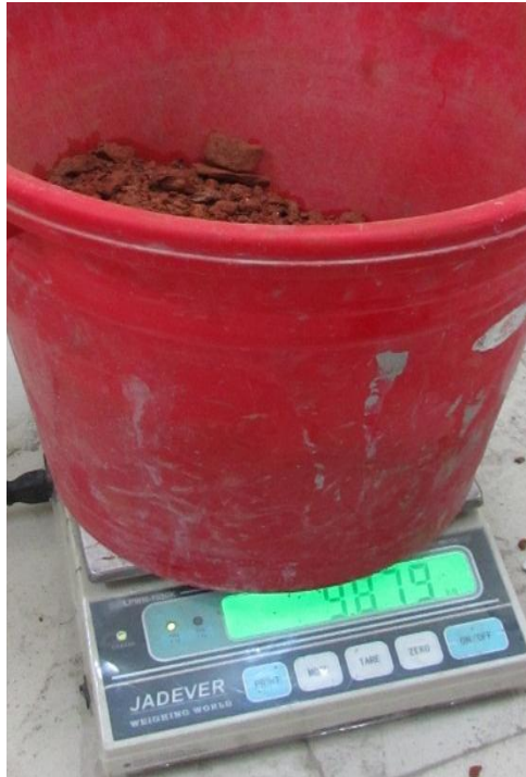
Figure 3.2 Measurement of brick chips
