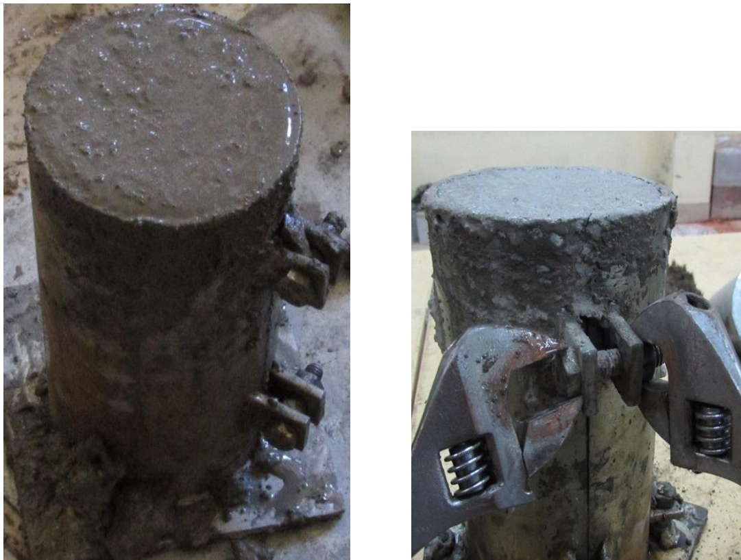
Figure 3.5 Casting and opening of concrete cylinder
