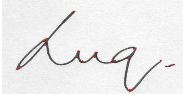
Figure 13: Keypoint detected (shown in red dots) in signature using Harris corner detection method
